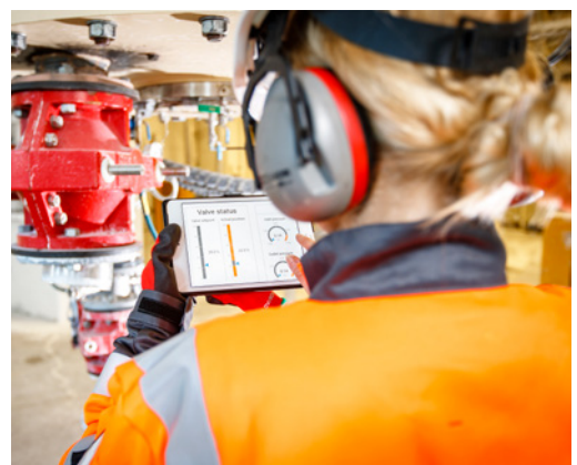
The Flowrox smart instrumentation can be retrofitted to automatic pinch valves.
