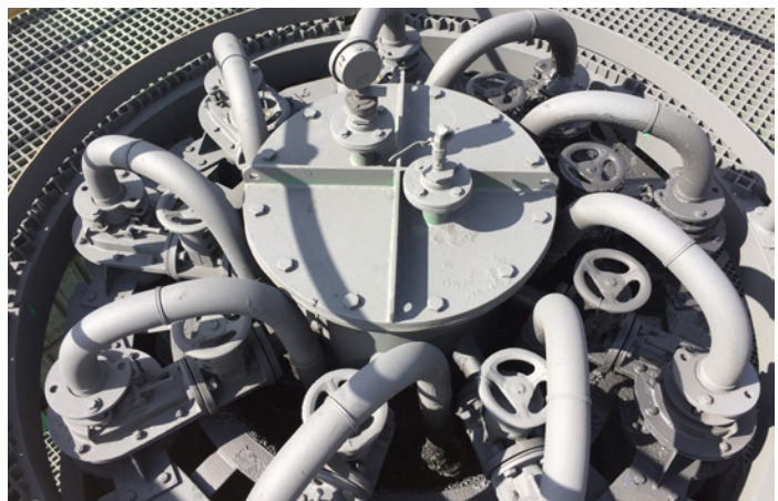
Image: PVEG50M manual polyamide body pinch valves in a hydrocyclone at Kara Mine, TMM, Tasmania, Australia.
