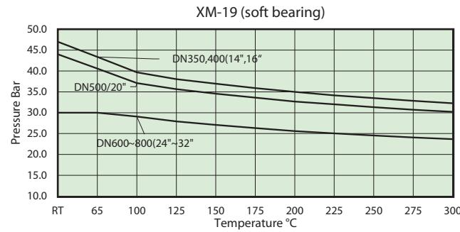
Max operating pressure differential in control service, RE
