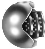
Liquid cavitation and aerodynamic noise problems can be solved with the patented Q-Trim™ valve trim. This design employs the two well-known principles of dividing the pressure drop into a series of small pressure drops and of separating the flow stream into many small jet streams. The use of these two principles combined with the rotation of the attenuator elements provides a combination of cavitation/noise abatement with high rangeability, high capacity and capability to handle impure fluids.
