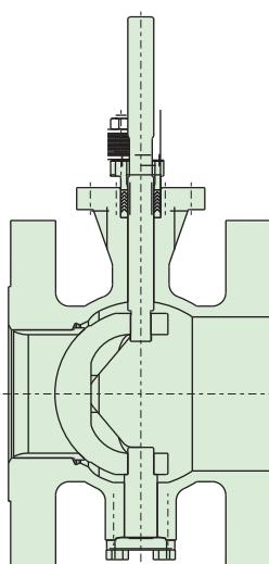
This heavy duty erosion resistant design handles contaminated flows and abrasive media at a favorable cost/useable life ratio. The seat is machined from cobalt chromium alloy and the seat design is changed from normal to reverse flow for maximum abrasion resistance. This version should not be used for isolation service since the seat is not in contact with the segment.
